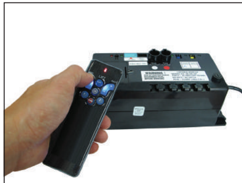
Figure 2: A flashing Green LED indicates the control box has received the remote control signal.
