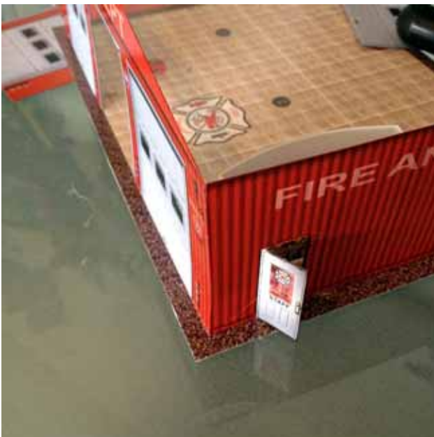
Figure 12 - Align and tack the walls using hot glue.
