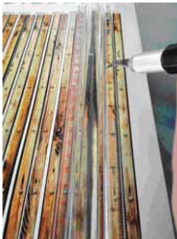
Figure 1 - Scoring the material.
