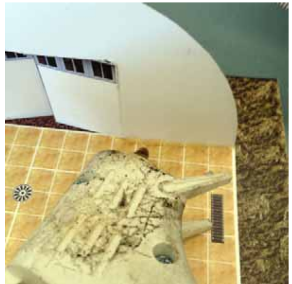
Figure 7 - Attach the front wall to the base using hot-melt glue.
