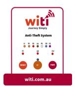
5. While the WiTi Wireless Communication Module is in PAIRING mode, retrieve the WiTi Wireless Brake Controller. Turn the ignition in the tow vehicle on to ensure there is power available at the 12V cigarette lighter socket. Press and hold the emergency Brake override button on the WiTi Wireless Brake Controller. While the Brake override button is still depressed, insert the WiTi Wireless
