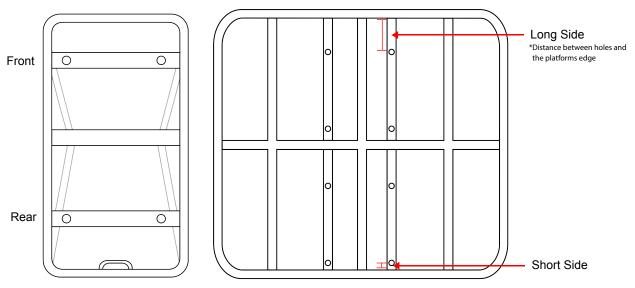
Attaching your platform to the front luggage rack: Your platform comes with offset holes, please note that the "short side" of the platform must be facing backwards allowing your platform to sit forward giving room for the electrical wires. Use four short allen bolts [A], eight washers and four nuts to secure to the front luggage rack. (no spacers required)
