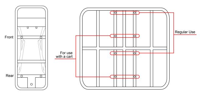
**Attaching your platform to the rear rack:** Your platform comes with offset holes, please note that the "short side" of the platform must be facing forward allowing your platform to sit back further, giving more room for the rider. Use four short allen bolts [A], eight washers and four nuts to secure to the front luggage rack. (no spacers required)
