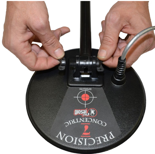
Figure 4 — Mounting Coil to Lower Pole
