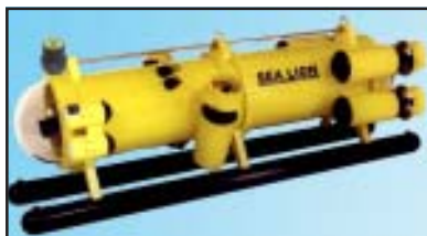
SCAN-650 scanning head mounted on Fishers SeaLion ROV.
