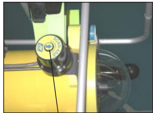
Mount Scanning Head arrow facing forward, this will be the top of the display on the PC
