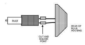
**CAUTION:** The bulbs should not be handled with bare fingers as oil from the skin gets onto the glass and will cause the bulb to burn up. If the bulb is handled with bare fingers, the glass should be wiped with denatured alcohol to remove any oil from the glass.
