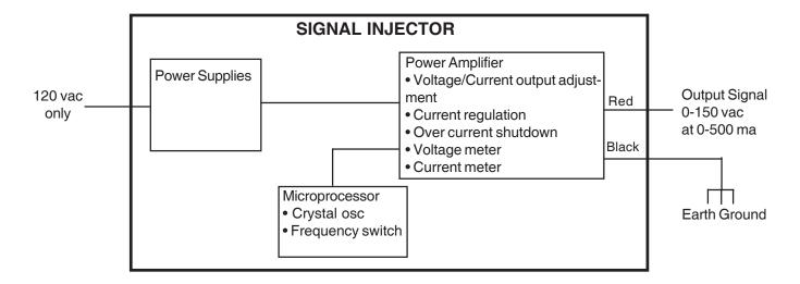
The Signal Injector contains a main logic board that has three main sections: Power Supply, Microprocessor, and Power Amplifier.
