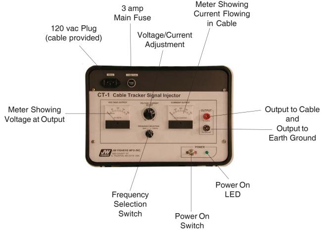
The control panel switches and indicators are:
