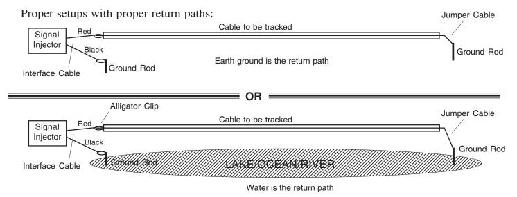
NOTE: Because water is a better conductor than earth ground, water as a return path allows higher currents to be put in the cable. However, since we need only 75-150 ma for most cables, earth ground works well in most cases. When earth ground doesn't do the job because the ground is very dry, a longer ground rod (deeper in the ground) can help.
