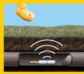
"I don't use a sonde often, but things went perfectly! We taped the sonde to a jetter and tracked it as it was fed down the line (which went under a business that was built over a section of the pipeline after it was laid). Once I pinpointed the sonde with the XT receiver, we further pinpointed it with the Schonstedt magnetic locator they already owned."
