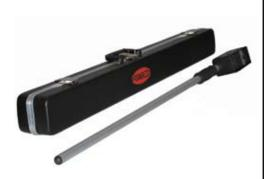
The Fisher FX-3 Ferro Probe senses fluctuations in the earth's magnetic field caused by buried survey markers, pipes, well casings, valves, iron relics, septic tanks and other ferromagnetic (iron or steel) objects. Because it's a differential-induction magnetometer, the FX-3 locates buried iron objects far beyond the reach of ordinary (search-coil-type) metal detectors.
