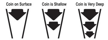
Objects other than coins will still register on the 3-segment depth scale, but the depth indication will be relative. For example, all 3 segments illuminated could indicate a coin buried 9" deep, but could also be a very large object several feet deep. Use the Depth Indicator in conjunction with the Conductivity Arc to gain more information.
