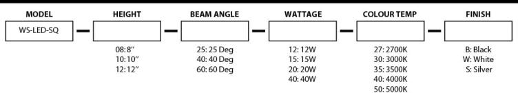
Example: WS-LED-SQ-08-40-12-35-B = WS-LED-SQ, height of 8", 40 degree beam angle, 12W, 3500K, black finish
