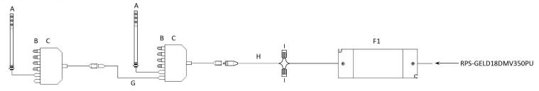
Max wiring distance between power supply and fixture is 20 feet. Up to six fixtures can be wired to a single distribution box (CC-6SP-500).
