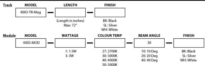
This fixture must be ordered as two components: 1. the track 2. the modules
