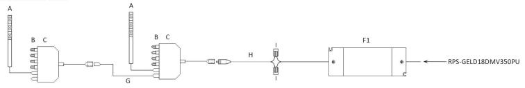
Max wiring distance between power supply and fixture is 20 feet. Up to six fixtures can be wired to a single distribution box (CC-6SP-500).
