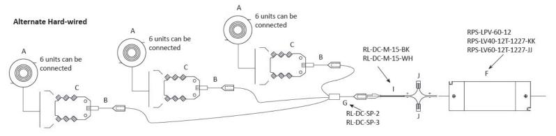
Max wiring distance between power supply and fixture is 20 feet (6m). Up to six fixtures can be wired to a single distribution box (CV-6SP-1224)
