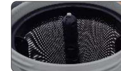
CHEMICAL CONTAINER RINSE NOZZLE
