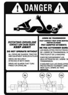
Label on outer protective tube
