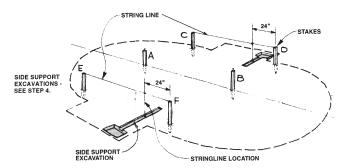
Locate stakes C, D, E and F from your pool layout. Attach strings between C and D, then E and F. Locate center of two side support excavations as shown. Other supports will be located 48" on centers if you desire to excavate at this time.
