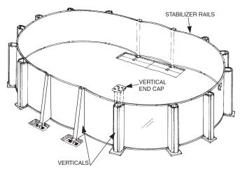
Carefully follow the detail in the exploded view to attach the verticals to vertical end caps to pool. Refer to your Pool Parts List exploded view when assembling verticals. Attach vertical at bottom first. Push vertical against wall, slip vertical end cap over wall and attach to vertical. Make sure vertical is straight. Attach other hardware as required in exploded view. Use all necessary hardware. Exploded view - Refer to Parts List for more detailed view. Fig. A
