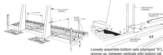
Dig out a trench to the dimensions shown above., grading to the ground support. Use a large screwdriver to scribe grooves (approximately 1" deeper) down each side and center of the trench to accomodate the pressure pads' flanges. Remove the excess dirt accumulated from scribing.
