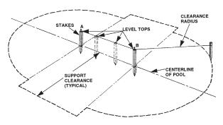
Locate stakes A and B. Level tops with long 2" x 4" board and carpenter's level. Layout clearances as shown. Remove all sod within pool area. This sod may be saved for future landscaping needs.
