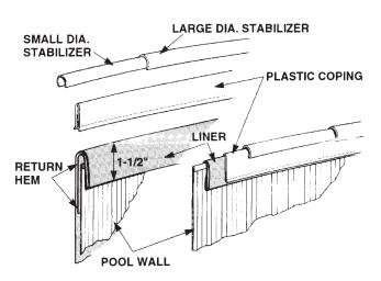
Make a return hem as illustrated. DO NOT cut off excess liner material as the liner will "Slip" from under the plastic coping, causing liner to fall back into the pool. Smooth liner against wall and secure to top of wall with plastic coping. Place stabilizer rails over coping, alternately telescoping small diameter into large diameter about 6 inches as before. One large diameter stabilizer rail fits between each pair of side supports. They DO NOT telescope.
