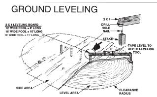
Using a transit to level the pool area is preferred. When using this method, professional assistance is recommended.
