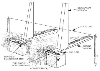
Remove string line. Place concrete blocks into the excavations as shown. NOTE: The thicker wall side of the cement blocks must face up. Level the blocks in both directions. Place the assembled side supports into each trench with skid plate resting firmly against the face of the concrete blocks. Check each ground support for level.
