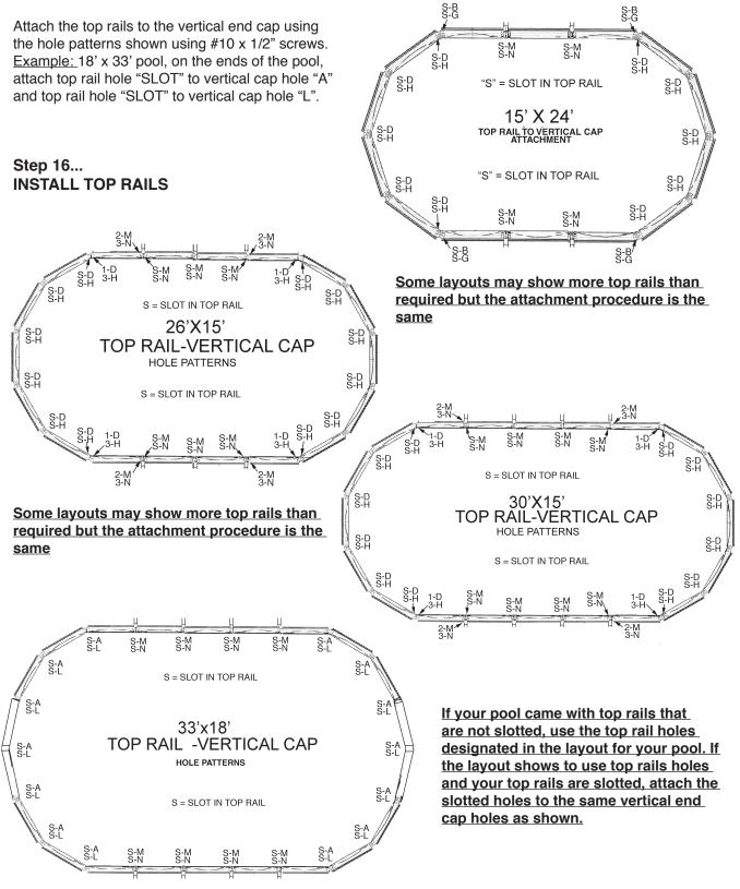
There are several different joints where top rails meet as shown. Refer to diagram for attachment and proper placement. Use four #10x1/2" screws to attach the top rails to the end caps.
