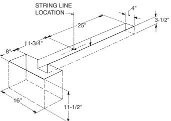
Carefully dig out side support trenches following dimensions above. Dig out side support trenches for the amount of side supports for your pool, refer to pool layout. It is very important that the trench walls remain firm and undisturbed during and after excavation. DO NOT over-excavate with the thought of back-filling later as the side supports will move when pool is filled and pool failure may result.
