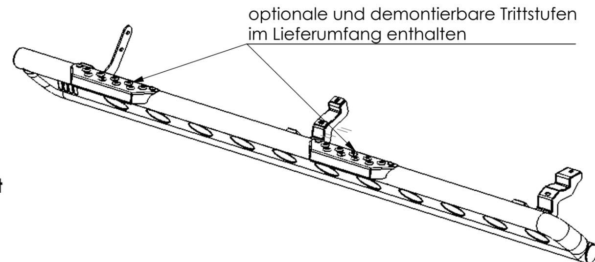
**Material: Slider Panele Aluminium, Halterungen Stahl**
