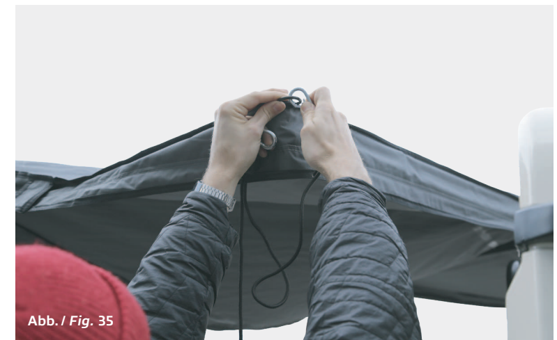
Markisenspanner in D-Ring / Awning tensioner in D-ring
