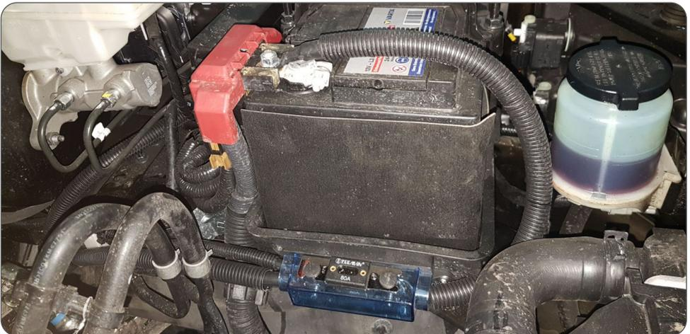
Route the cables from the loading bed in the underground of the car to the battery case. Ensure that you route the cables with existing cables that are properly protected. Fixate fuse near battery and connect the system to the cars battery. Use zip ties to fixate cables.
