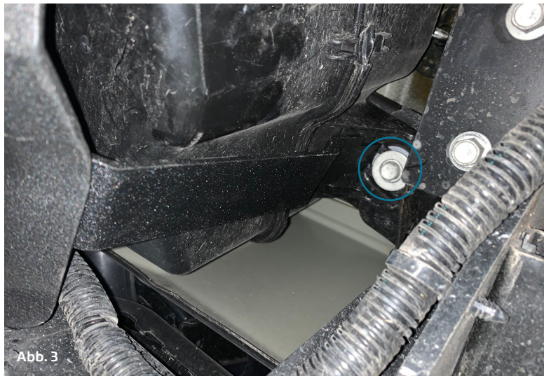
Montagepunkt hinten links / mounting point rear left
