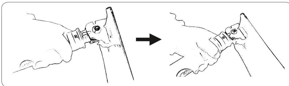
Holding spring sleeve and pulling back, turn the shovel head down and fixed at the fixing groove, then release the spring groove. Shovel head is fixed at 90 degree.
