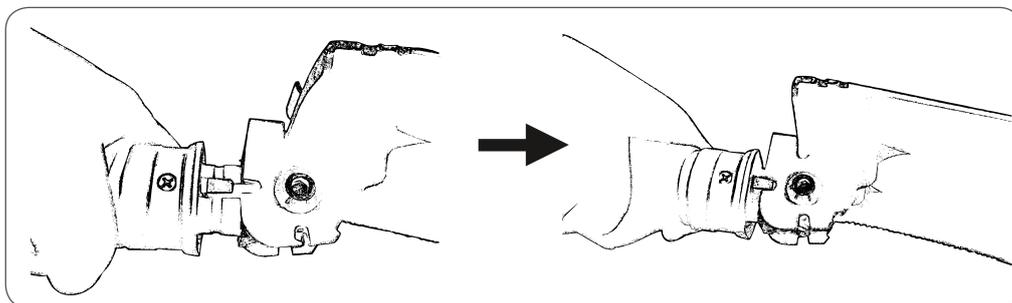
Holding spring sleeve and pulling back, turning the shovel head up to the fixing groove. Then release the spring sleeve. Shovel head is fixed at 180 degree.
