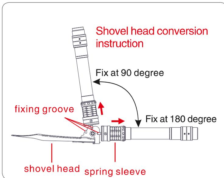
Pulling spring sleeve back and then the shovel head can be fixed on the fixing groove. When shovel head is fixed at 90 degree, it can be used as hoe. When shovel head is fixed at 180 degree, it can be used as shovel.
