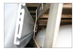
You can fix the awning on a vertical surface by simply drilling 4 holes with the disired distance and use the sliding bolts to fix the awning directly to your car/basket. Check the intergrity of the surface you plan to mount the awning to first.
