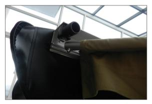
Feed the transverse pole into the sleeve till the other head outcrop.
