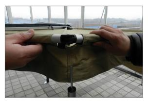
Aim at all lognitudinal pole and transverse poles holes. It need force to tighten the fabric.
