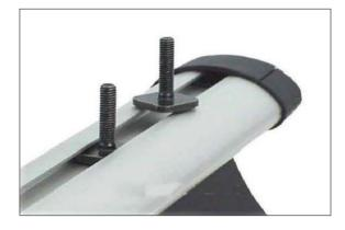
Many roof racks have a mounting track system that allows to use sliding bolts to fix the L-shaped brackets.
