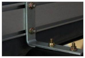
Make sure the sliding bolts have necessary size(M6) to fit the mounting brackets. Position the brackets on top of the rack and fix them with washer, split ring and nut.
