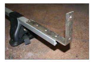
You can adjust the height by installing the brackets facing up or downwards.
