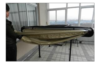
Unfold the awning slowly and stop in first triangle unfolded completely, meanwhile hold the other part of the awning.
