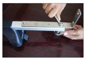
Fix the L-shaped bracket to your rack by using M6 bolts at the necessary length and tensile strength.
