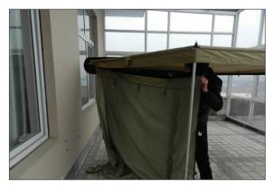
Fix the awning wall and awning with velcro. Paste wall and awning together .
