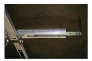
Drill at least 2 holes for each L-shaped bracket. We highly recommend to take the racks off your car for this procedure.
