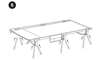
Put one end of the support rod on the crossbar, clamp it down and lock it as shown above. Then do the same to the other end.
