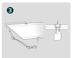
Unfold leg frames and click to secure. Attach leg frame brackets to side rails. Align all the tensioning levers on one side. Set the cot on its side, levers facing up, and apply pressure to lock the levers into position.
