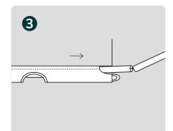
Remove the side rails from the pockets of the fabric top. Slide to separate and fold.
