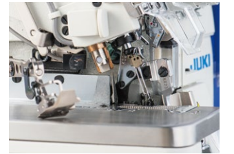
3. Presser foot arm with an open/close sensor
