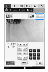
Press the positioning keys to move the embroidery frame until the thread mark on the fabric is aligned on the starting point in the camera view window.
