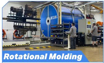
Complex shapes that allow for our tank designs are best achieved with in-house equipment. We own multiple dual station rotational molding machines that allow us to produce finished parts from raw plastic. Producing consistently higher quality parts, and respond quickly to sales spikes.
