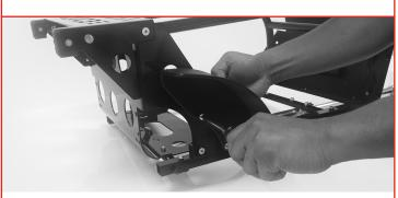
6. Line up the lower hole in the fender with the nut inside of the fender lock. Use a 16mm bolt to secure. Tighten fully and then tighten the bolt from Step 4. 7. Repeat Steps 1-6 for the alternate fender.
