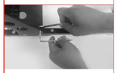
3. Remove the top bolt that attaches the side panel to the square tube. You will not need this bolt, but set aside the nut for Step 4.
