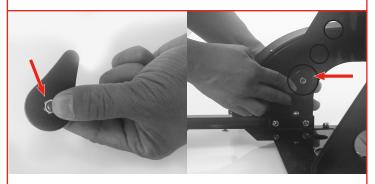
5. Snap a 10mm nut into a fender lock.
