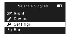
In the Settings Menu, Sound can be enabled/disabled and the Polarity of the CELLER8® products can be altered.
