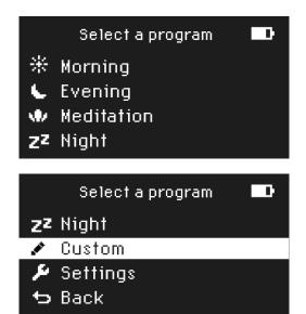
To return to the Application Menu, use the Control Dial to scroll to *Back* and press the Control Dial to return.
