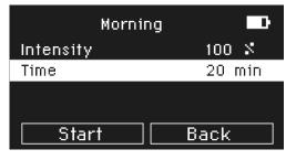
Turn the Control Dial to adjust the Time as desired. Press the Control Dial to confirm.
