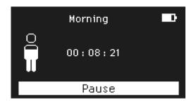
To pause the program, press the Control Dial; press once if the screen is active, or twice if the screen has dimmed. A prompt will appear giving the option to Stop or Resume the program. If the program is to be resumed after a break, use the Control Dial to ensure Resume is highlighted and Control Dial to resume the current session.
