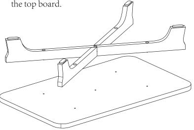
4. Align the leg board screw holes and the top board screw holes to drive in the other 4 screws.
