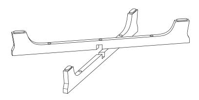
3. Drive the 1st screw into the leg board center screw holes and top board center screw hole to lock them together.
