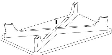
2. Put the leg boards onto the stand top board, aligning the screw holes in the leg boards and the top board.
