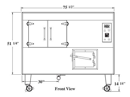
**Note:** When purchased with a VSP Hood System the caster legs are replaced with 19" working height legs (no casters) New overall working height of the oven with legs is 70.25"
