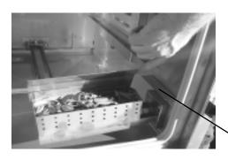
4. Next remove the chip box by sliding it off the element support. Fill the chip box with chips and place it back over support bracket. Make sure the lid is closed and slide the chip box all the way to the right under the drip edge.
