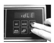
2. Press the arrow Up or Down button until the desired menu is displayed. There can be 40 programmed menus stored on the controller.
