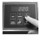
8. Press the Up or Down arrow to set the desired cook time for step 1.
