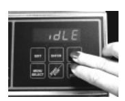
2. Press the arrow Up or Down button until the desired menu is displayed. There can be 40 programmed menus stored on the controller.
