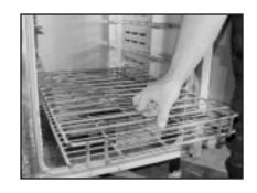
2. Lift the steam diverter from over the steam pan located in the bottom of the oven.
