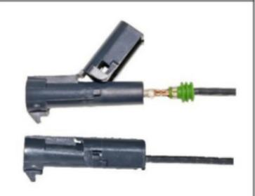
Completely close the jaws to crimp the terminal to the wire. Insert the terminal and seal into the seal die and crimp the terminal to the seal. Pull test to ensure a complete crimp. Insert the terminal into the connector until it clicks.
