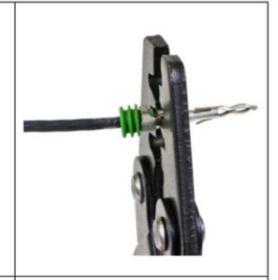
The CT-18 tool has five dies for 1. crimping a variety of terminals and seals 24-12 gauge. Use 2. this chart to locate the correct dies for your intended use.
