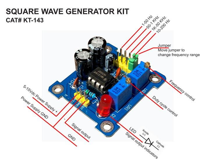
PC board is clearly marked. Observe polarity when positioning electrolytic capacitors and LED. Long lead of LED is anode (+). Solder 8-pin IC socket in place before inserting 555 timer. Little semicircle on pc board, in socket and 555 timer should face the same way. Break 8-pin header strip into two 4-pin pieces and solder in place. 2-pin jumper bridges these two headers and, depending on which are bridged, determines the frequency of the circuit.
