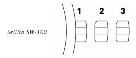
Be careful, do not use position 2, it could damage the movement.
