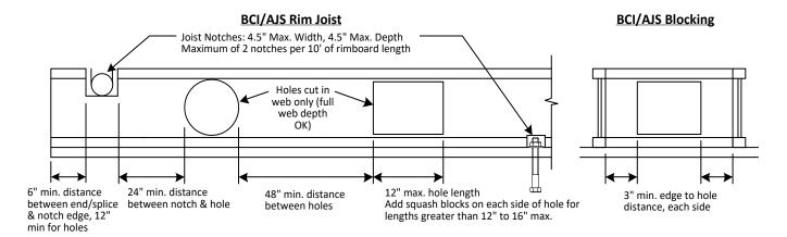
As required in all AJS/BCI rim joist and blocking applications, concentrated loads from king studs, columns, beams, and other sources require squash blocks to transfer the load away from the AJS/BCI product.
