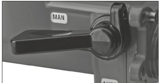
Fig.11 Particular of the "S" selector in "MAN" position.
