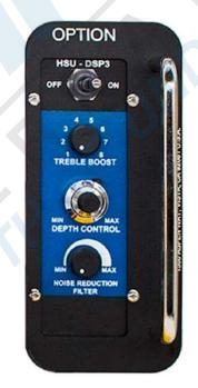
3.3.1 **ON/OFF SWITCH** – Allows the selection of air (OFF) or helium (ON) operation. In the OFF position, the divers' microphone signal bypasses the HSU. In the ON position, the microphone signals are routed to the HSU and the tender can adjust the controls as necessary.
