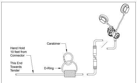
FIGURE 3: Recommended Setup of the Diver ComRope
