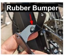
c) Slip the upper fender bracket onto the top of the lower triple tree. See photo below.
