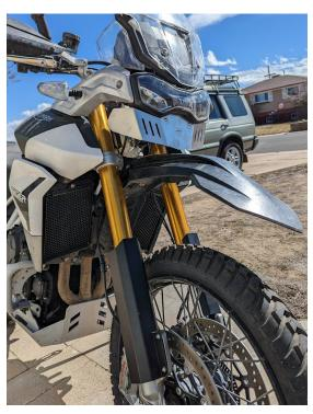
Conduct a final check to make sure all parts are fastened securely and that nothing will interfere with the full travel of the forks (Brake line slack length and fork guard placement) or lockout of the handlebars in both directions.
