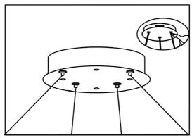
5. Adjust the steel cable length and balance of the lamp body with the adjuster on the chassis
