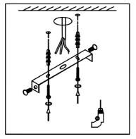
1. Install the hanging plate on the ceiling with 2. Connect the wires of the LED driver to wood screws or expansion screws
