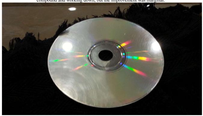
Lay the CD flat on a cloth, and use the same small circular motion and work your way around the CD. Don't be afraid to use a lot of pressure. In this picture, the right half is polished, and the left half is still 5,000 grit sanded. After polishing the whole CD, finish with clear plastic polish.
