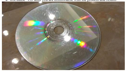
My test CD was in pretty bad shape, having spent most of its life out of its case, in the accessory pocket of my mother-in-law's 1995 Honda with a stack of other CDs. It was semi-playable, but had noticeable distortion and noise. Notice the ring around the outside from spending some time in a CD wallet.
