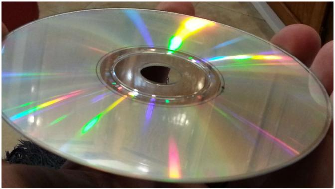
CD after polishing with glazing compound and clear plastic polish. While some fine circular scratches will still be visible in direct light, they don't seem to affect the playback in any way. This CD played perfectly and the noise was gone!
