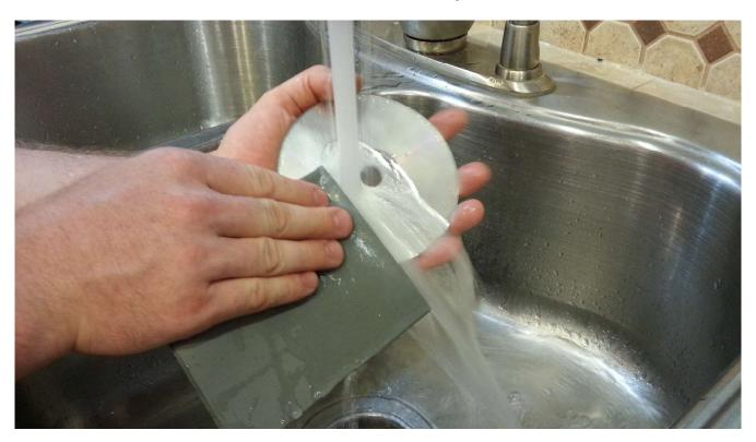
Fold the sandpaper in half, and wet-sand the CD under running water. Use a small circular pattern, and slowly work your way around the CD's surface to remove any deep scratches. Use the palm of your hand to keep the CD from bending too much, and to help get all the way to the outside edge.
