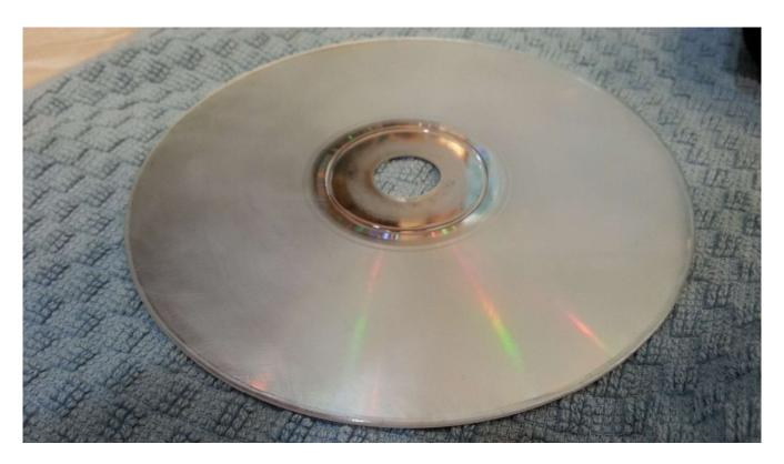
After the 2000 grit, the surface should be dull and evenly "scratched". If you see any deep scratches that stand out, keep sanding! Notice how the light/rainbows don't reflect very well anymore.
