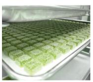
Gummy curing (drying) is a critical step in the gummy production process. It is of great importance to dry your finished gummies to the target moisture level to ensure their optimal texture and stability.
