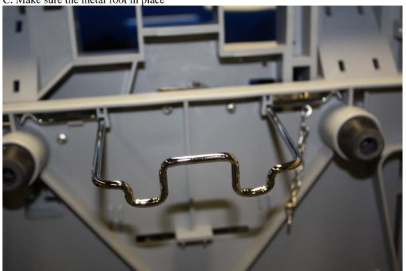
D. Fold the metal foot below the oscillation plate
